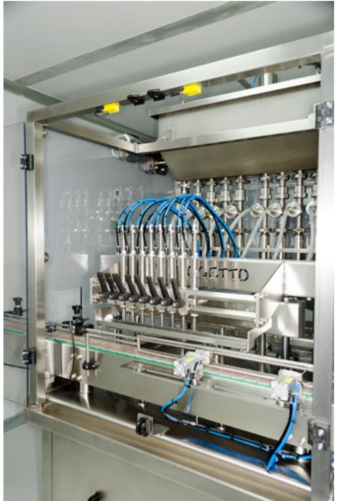
The liquid filling machine for oral medicinal syrups and other liquids.
