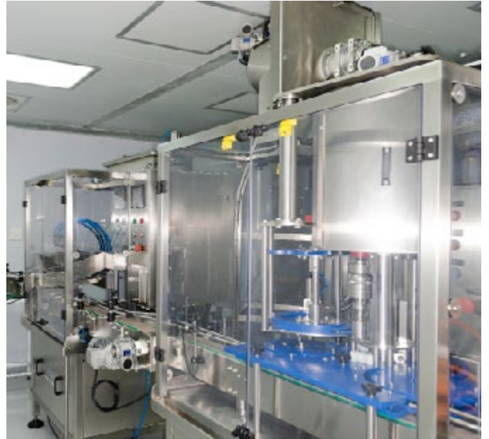
The liquid filling line.
